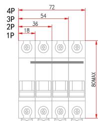
Installation guide rail dimension diagram
